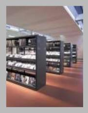
The shelving system structure is based on separate suspension of the many different components in rows of holes at 25 mm intervals, punched out in freestanding single- or double-faced uprights and wall strips.
